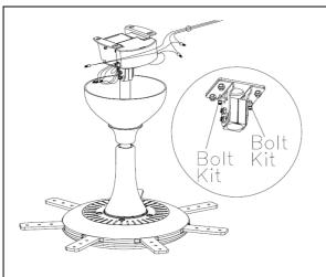
9-1 Loosen attach bolt kits on fixed bracket, raise the canopy, then secure it to the fixed bracket.
