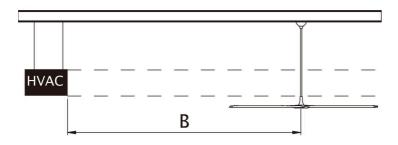
B: The distance between the center of the ceiling fan and HVAC equipment need to at least 2x diameter.
