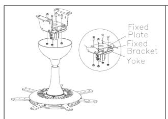
\* Make sure the extension tube unit with the horizon is 90 degrees.
