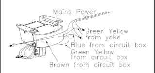
\*As shown in the figure, after the wiring is completed, the live wire (L), the neutral wire (N) and the earth wire (E) should be at the both side of the Circuit Box.
