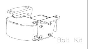
8-1 Loosen and use bolt kit of the yoke. Secure the circuit box's earth wire with the yoke.
